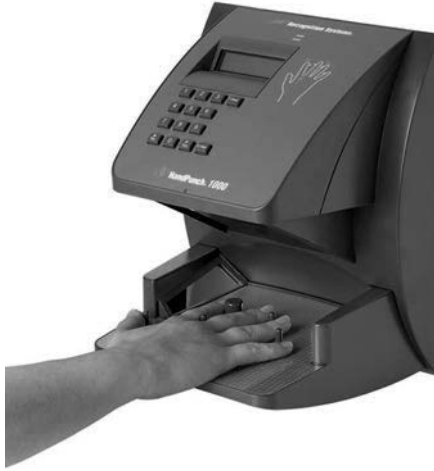
Resim 7.4: El geometrisi temelli bir güvenlik sistemi (Kaynak: Pearson, R.L. (2007). Electronic Security Systems: A Manager's Guide to Evaluating and Selecting System Solutions, Butterworth-Heinemann, Elsevier).
